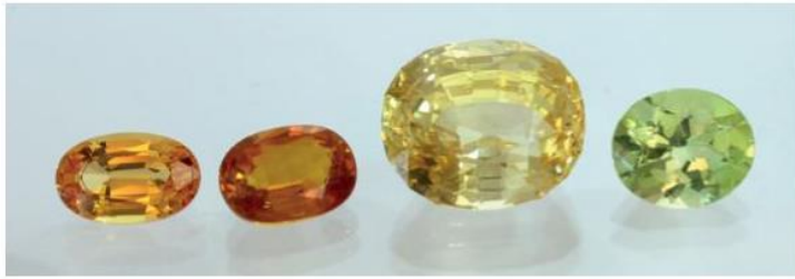
4: Yellow stones. Penetrating up to 7mm from any surface, beryllium diffusion can affect the colour of an entire stone or just a shallow surface layer. Colour of beryllium diffused yellow sapphire is often a deep golden or greenish yellow, but every shade of yellow has been seen, including pastels. Shown are various shades of both untreated and treated stones. Learning which is actually which treatment category may be surprising.
