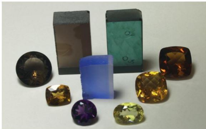
6: Quartz. Artificial colours that test as quartz make for an easy ID, but there is no variety nor shade of colour seen in natural quartz that has not been synthesized, including inexpensive smoky quartz and lemon quartz. More batch testing at the dealer and manufacturer level would increase confidence in the market.
