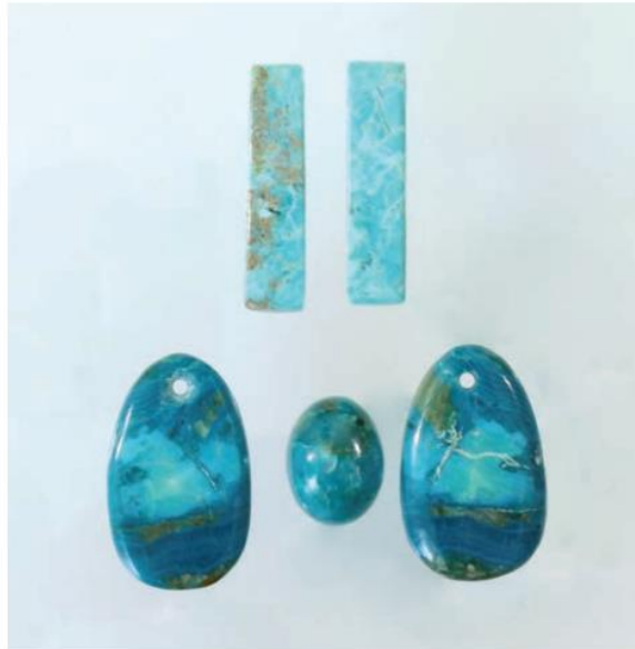
Figure 7: These polished samples consist of Apache Blue Stone that has been stabilized by polymer impregnation. The pieces on top (23.4 × 5.6 mm) were treated by the currently used stabilization method, while those on the bottom (drop shapes of 22.0 × 14.0 mm and an oval cut of 12.3 × 9.4 mm) were treated by an older polymer impregnation technique that partially darkened their colour. Photo by Dean Brennan.
