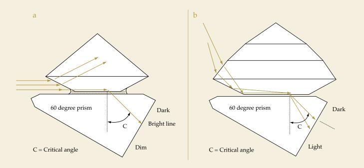
*Figure 6:* Sketch of the light paths in the prism of a gemmologist's refractometer when grazing incidence is used. In position (a) light is directed in the plane of the prism surface. In position (b), light is directed into a pavilion facet from above and behind.
