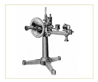
*Figure 3:* Pulfrich refractometer, catalog scan taken from Arthur H. Thomas Co. Laboratory Apparatus and Reagents. Philadelphia (1921).
