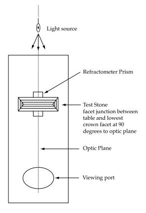
*Figure 7:* Diagram of a refractometer showing the placement of a gem with respect to the optic plane of the refractometer.
