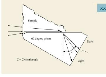
*Figure 4:* Sketch of the light path in the sample and prism of a Pulfrich refractometer when solids are measured.
