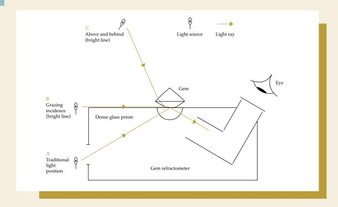
*Figure 5:* Diagram of a refractometer showing the positions *a*, *b* and *c* of a light source for traditional illumination, and for grazing incidence.
