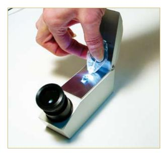
*Figure 2:* Modern style refractometer with small LED light directed at grazing incidence.
