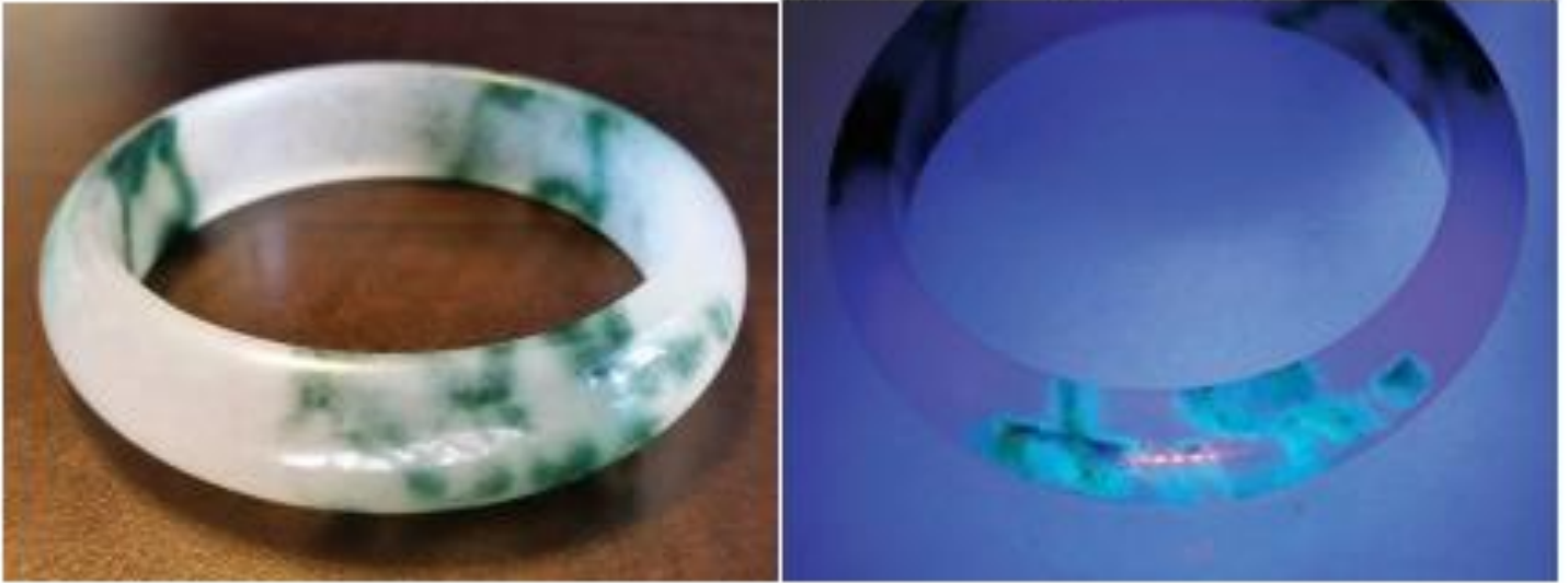
Figure 27: Although appearing like 'moss-on-snow' jadeite, this 16.9-mm-diameter bangle consists of dyed quartzite (left). The green areas of the bangle exhibit strong green fluorescence to long-wave UV radiation (right). Photos by B. Williams.
