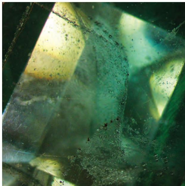
Figure 21: Microscopic examination of the green glass revealed straight and curved planar arrangements of gas bubbles. Photomicrograph by B. Williams; magnified 20×.
