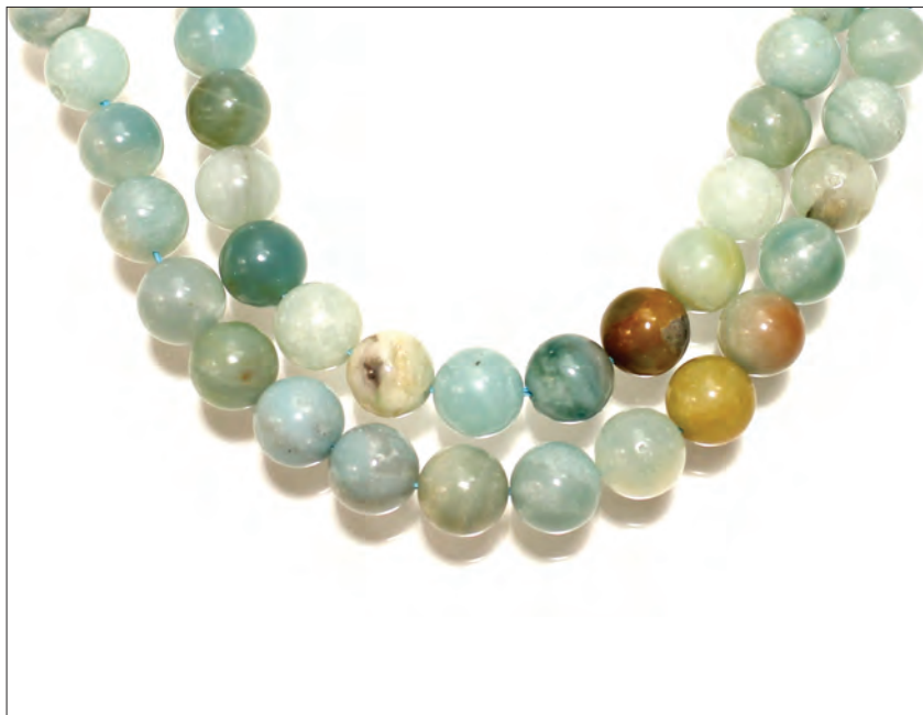
Figure 33: The wide variation in colour and pattern seen in these 12 mm beads provided a strong indication that they were not amazonite. The beads proved to consist of chalcedony and quartzite, most of which had been dyed. Photo by B. Williams.
