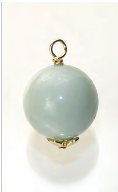
Figure 32: This 'amazonite' earring (16 mm in diameter) was found to consist of dyed quartzite. Photo by B. Williams.
