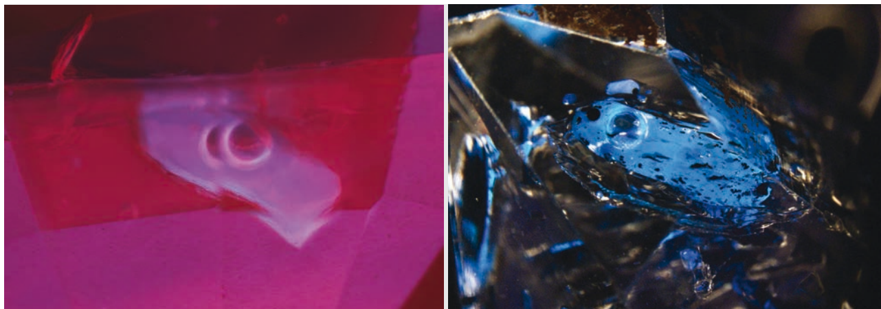
Figure 28: Left: Under long-wave UV radiation (365 nm), the petroleum exhibits a chalky blue-white reaction that was somewhat muted by the dominant red luminescence of the host spinel. Right: Such fluorescence also is displayed by petroleum inclusions in a Pakistani quartz. Photomicrographs by C. P. Smith; magnified 40 \times .
