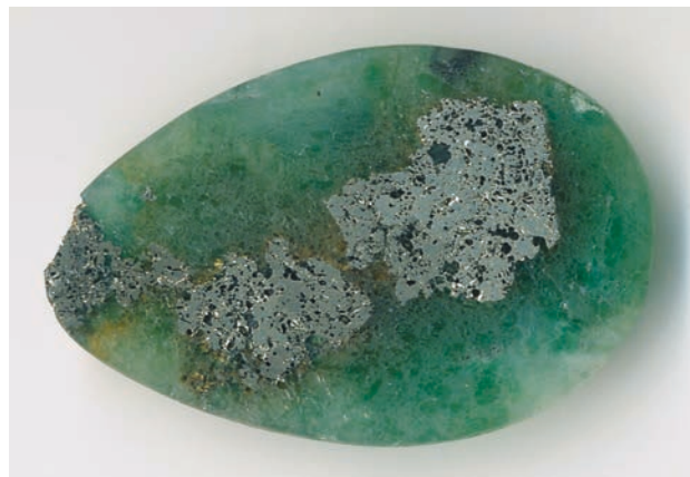
Figure 9: The texture of the various minerals is visible on the base of this cabochon (35 mm long), which shows irregular corroded masses of pyrite and granular intergrowths of emerald and dolomite. Photo by J. Hyršl.
