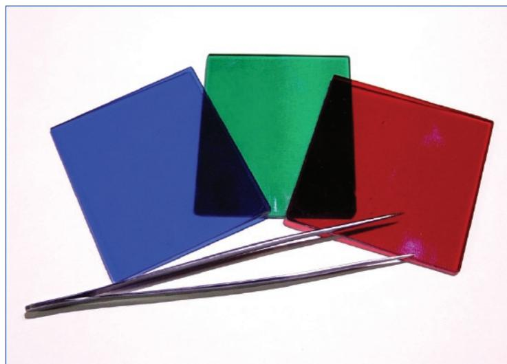
**Figure 2a:** Photograph of the glass filters used in this investigation with gem tweezers for scale.
