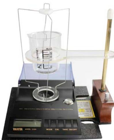
By popular demand, Gem-A Instruments is now stocking a Specific Gravity Kit. This simple but effective test can help to identify stones when all other tests are inconclusive.
