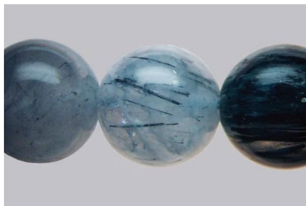
Figure 30: The surface-reaching inclusion in the bead on the left was found to consist of a hollow etch channel that contained coloured resin. In a few of the beads, the coloured polymer also penetrated surface-reaching fissures, as shown on the right. Photos by C. Williams; both beads are 10 mm in diameter.
