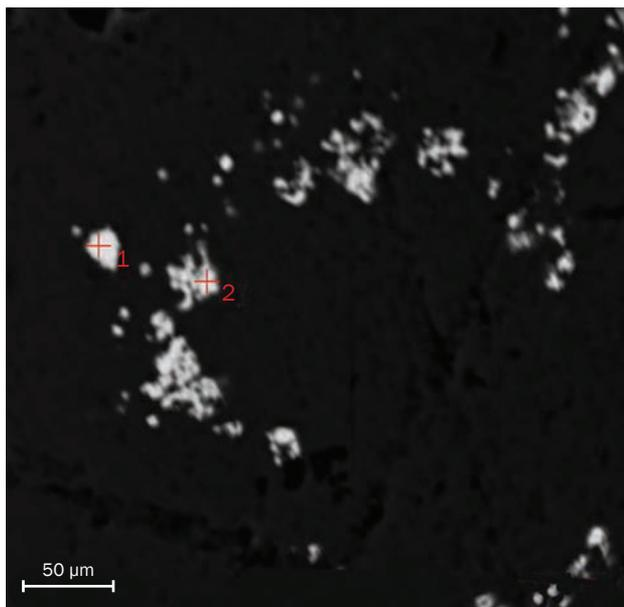
Figure 13: Backscattered-electron imaging of a polished surface of Utah Lace Opal shows bright-appearing sulfide inclusions. Approximately 20% of them consisted of an unidentified antimony thallium sulfide (e.g. spots 1 and 2), and the remainder were pyrite or marcasite. Image by A. U. Falster.
